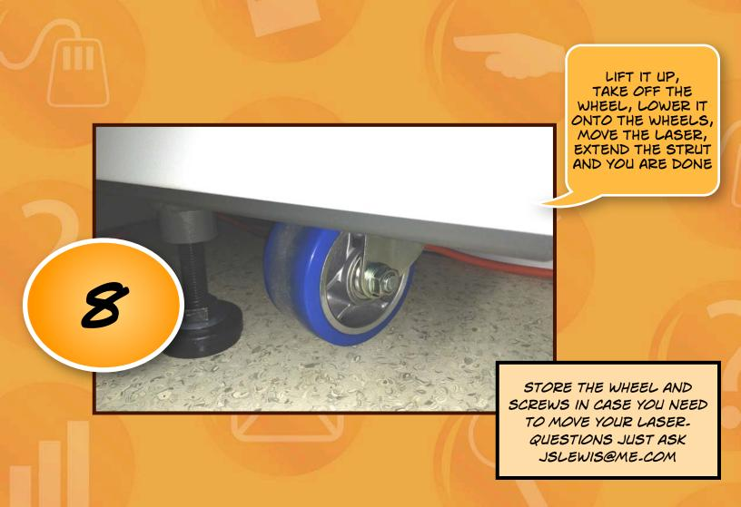
Use a wrench to lift the NIDEK off its wheels by turning the struts. The struts will extend very easily. Remove the wheel nearest the VISUMAX. Next. retracted the struts so the NIDEK rests on 3 wheels. My wife pushed down on the opposite edge of the NIDEK for balance and I moved the machine about 6 inches into the position shown above. I extended the struts again and lifted the NIDEK off its wheels and into its final position. Checked the NIDEK with a level and was done. Five minutes max.
